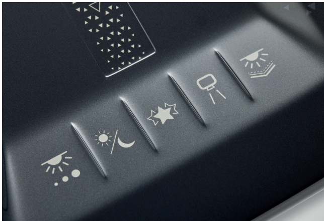
Fig. 1. The organic 3D shaping of the surface supports the intuitive operation of the touch buttons. © Leonhard Kurz
